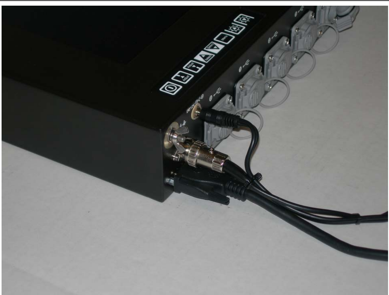
Figure 1-6 Cable connections and cable ties in front view
