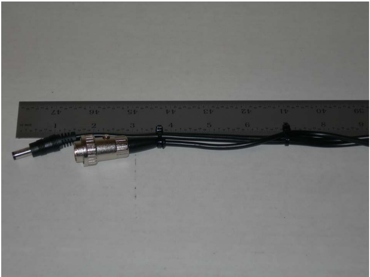
Figure 1-4 Excess Tie material removed
